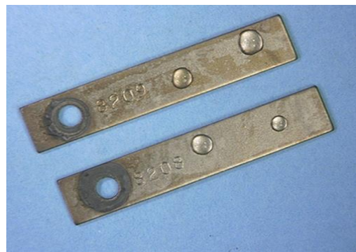
Figure 1: Water beading on LCS coupons following Polyamine treatment
